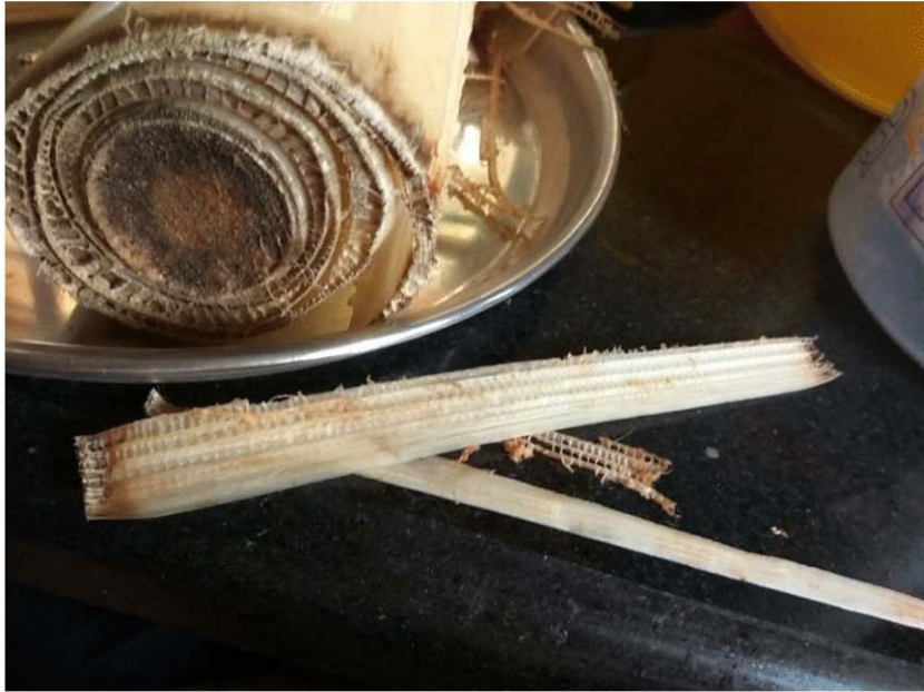
Banana stem peeled in three ways- *Gridded skin (water content); just the grids layer; dry fibrous skin
