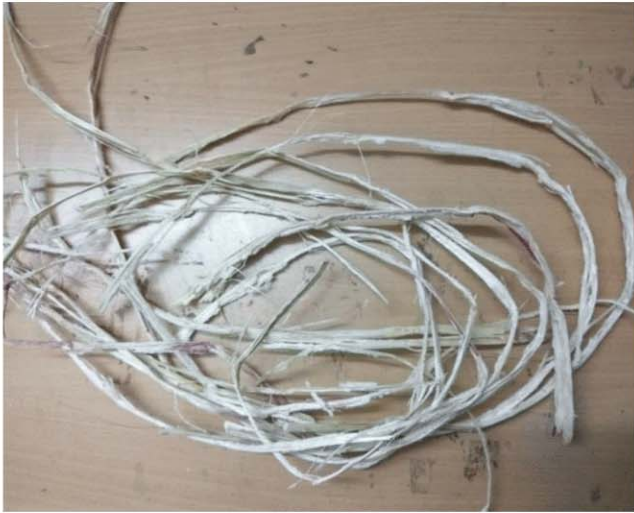
Soaked sugarcane waste strands into palm leather solution (20 % glycerine and 80% water) for 6 hours and then let it dry in shaded sun.
